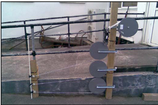
Fig 6: Example of a retractable electric fence system.
